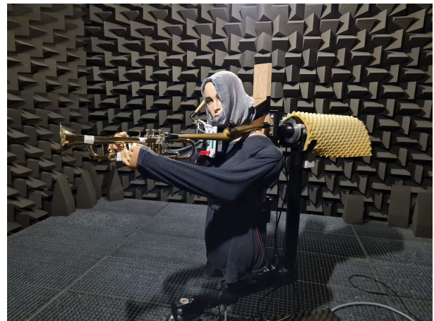
Figure 1: Setup used for the measurement of a trumpet in 3D measurements with a mannequin and a turntable.
