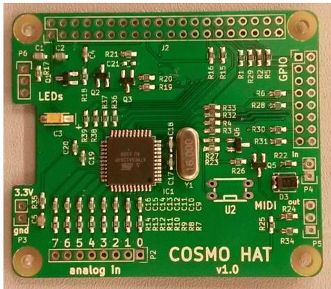
Figure 2: COSMO-HAT circuit board to connect 8 analogue controller inputs, 8 LED's or switches and MIDI I/O.
