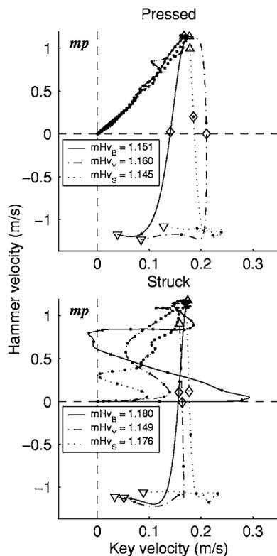
FIG. 2. Touch trajectories of *mezzo-piano* keystrokes at the C5 (72) on three pianos played with pressed touch (upper panel) and struck touch (lower). Upward-pointing triangles denote escapement point, diamonds hammer-string contact, and downward-pointing triangles key bottom contact times. Small filled circles are plotted on the trajectories every 2 ms to indicate time.
