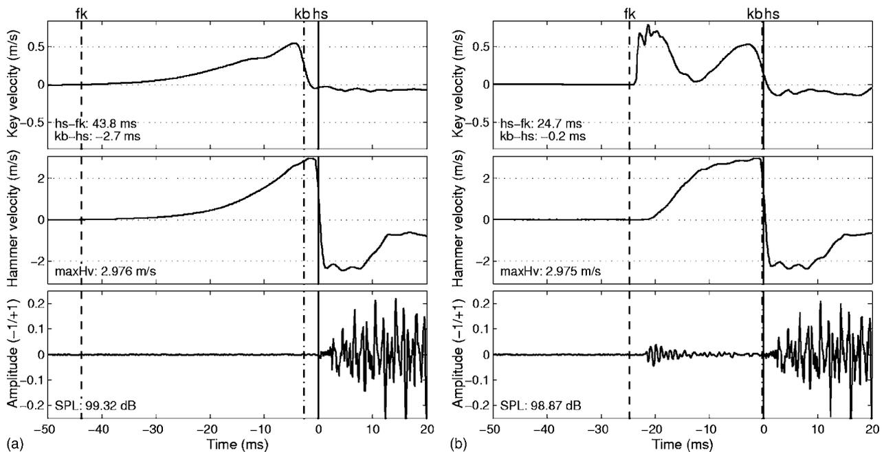
FIG. 1. Two *forte* keystrokes (C4, 60) played on the Yamaha grand piano with a pressed touch (left) and struck touch (right). The top panels show key velocity, the middle panel hammer velocity, and the bottom panel the amplitude of the sound signal. Both keystrokes exhibit similar MHVs and peak sound levels. Finger-key contact time (“fk”), hammer-string contact (“hs”), and key bottom contact (“kb”) are indicated by vertical lines.
