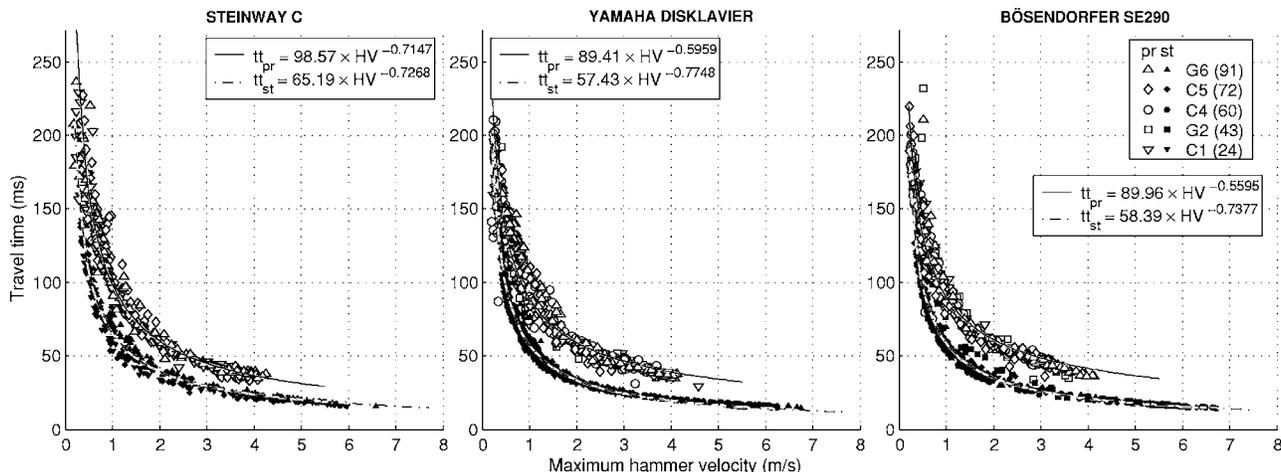
FIG. 6. **Travel time** (from finger-key to hammer-string contact) against MHV for the three grand pianos (three panels), different types of touch (*pressed* and *struck*), and different keys (from C1 to G6, see legend). The two types of touch (“pr” and “st”) were approximated by power functions (see legends).
