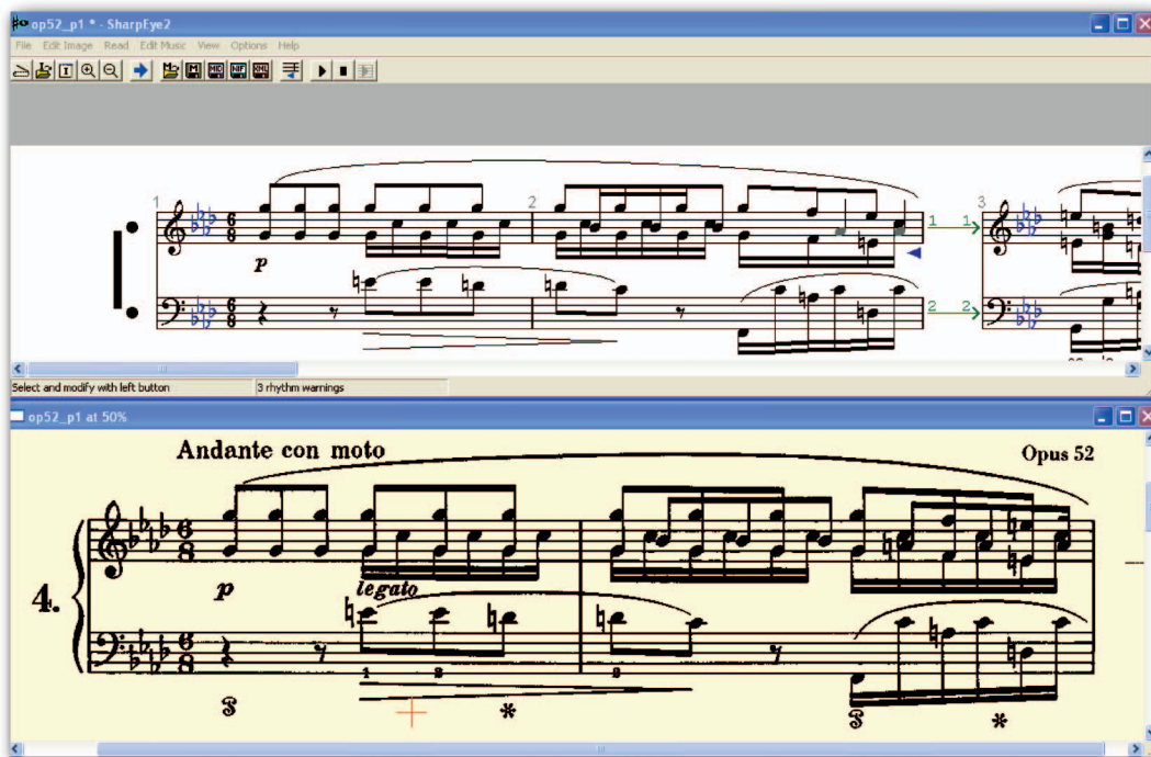
Fig. 1. The SharpEye OMR Software showing the printed score (lower panel) and the result of the recognition software (upper panel).
