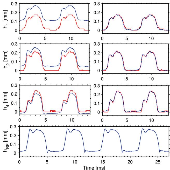
**Figure 3.** Reed-tip openings obtained after fitting the strain signals (blue) and their corresponding HS-camera signal (red), for measurements 1, 2 and 4, using the fitting model 3 as a reference. At the right, the calibrated signals (blue) are obtained after adjusting the reed-mouthpiece closure ( $h = 0$  mm). At the bottom, a calibrated real-playing strain signal, which cannot be compared with a camera signal.
