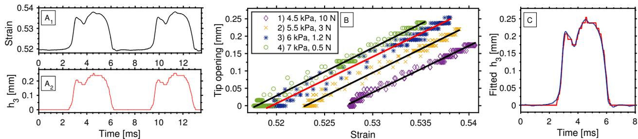
**Figure 2.** A: Original strain ( $\varepsilon$ ) and its corresponding reed-tip opening ( $h_3$ ) seen by the HS-camera for the measurement at 6 kPa and 1.2 N (label number 3). B: Reed-tip opening vs. reed strain at different pressures (kPa) and lip forces (N) and their linear fitting model; model 3 (red) is taken as the reference for the calibrated signals in Fig. 3. C: Reed-tip opening from the camera (red) over the fitted strain signal (blue) for measurement number 3.
