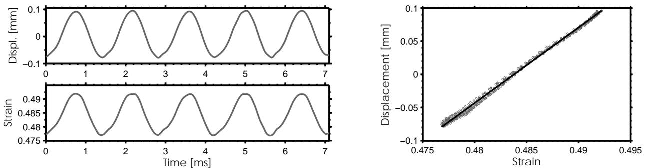
**Figure 4.** Evolution of displacement and measured strain (left) together with their linear correlation (right) for a vibration at 700 Hz (A in Figure 5) of the reed of strength 3 ½.
