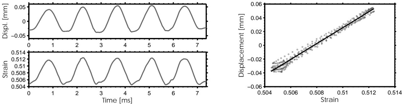
**Figure 2.** Evolution of displacement and measured strain (left) together with their linear correlation (right) for a vibration at 702 Hz (A in Fig. 3) of the reed of strength  $2\frac{3}{4}$ .
