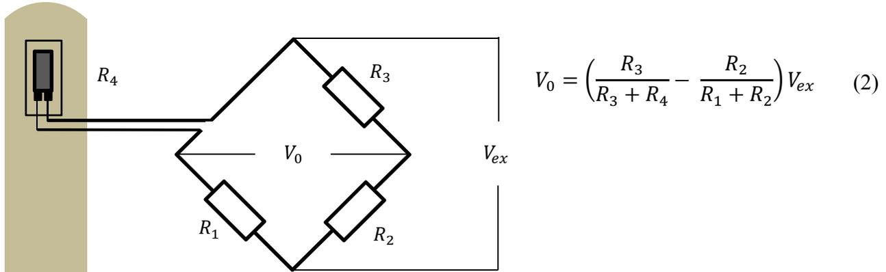
**Figure 6.** Quarter-bridge circuit with a strain gauge attached to the reed (adapted from [12]).
