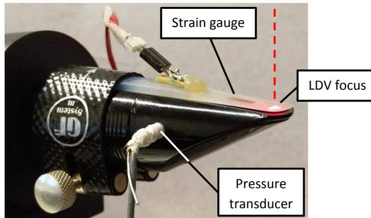
**Figure 1.** Setup with a strain-gauge sensor reed, a pressure transducer inserted to the mouthpiece and the LDV focus point at the reed tip. The vertical dashed line indicates the direction of the LDV light beam.
