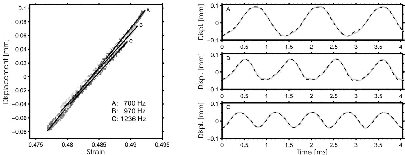
**Figure 5.** Strain-displacement fits for the reed of strength 3 ½ at three frequencies (left). Corresponding displacement signals (right) of the mapped strain-gauge (dashed black) compared to the original LDV (grey).
