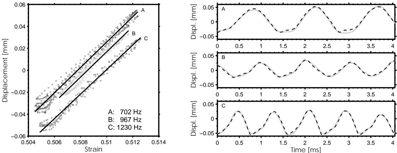
**Figure 3.** Strain-displacement fits for the reed of strength  $2\frac{3}{4}$  at three frequencies (left). Corresponding displacement signals (right) of the mapped strain-gauge (dashed black) compared to the original LDV (grey).
